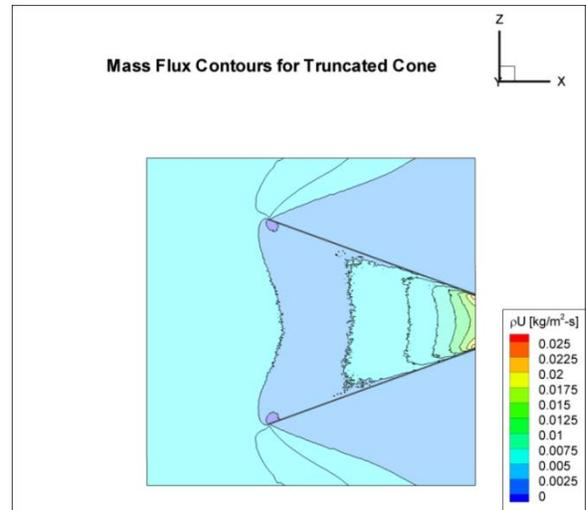
Figure 6--Mass flux contours for truncated cone.
