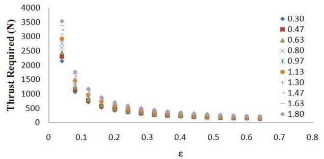
**Figure 9--Thrust required as a function of  $\epsilon$  (x-axis) and  $C_{D, \text{geom}}$ . (markers). Thrust requirements decrease as  $\epsilon$  increases.**
