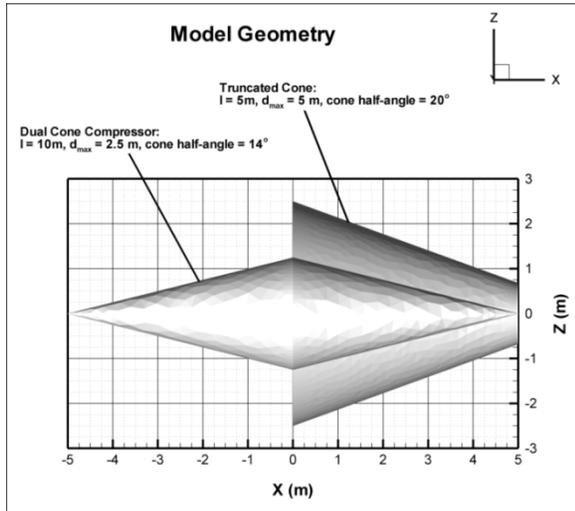
Figure 3--Inlet geometry with dual cone compressor.
