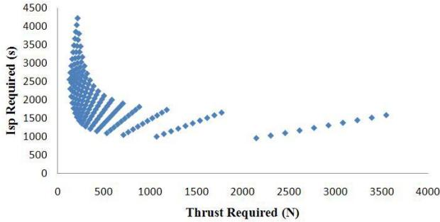
**Figure 10--Spread of Isp and thrust requirements for Mars mission. Minimum performance requirements cases are in the lower-left corner of the plot. The spread results from the range of  $C_{D,geom}$  and  $\epsilon$  values considered.**
