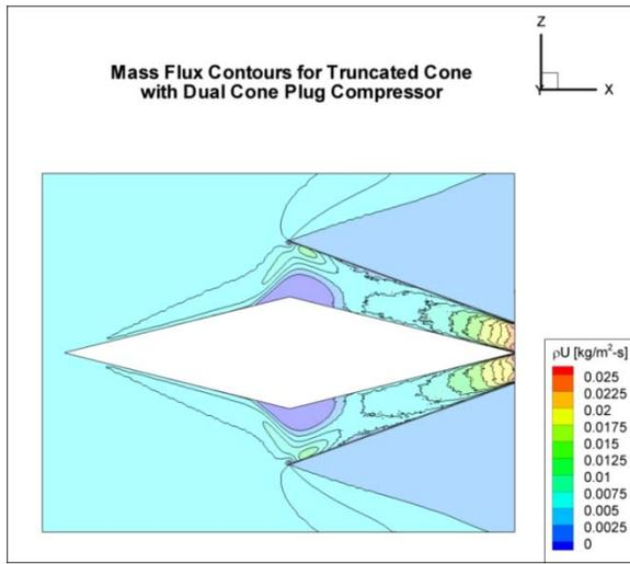
**Figure 7--Mass flux contours for truncated cone with compressor.**
