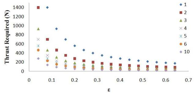
**Figure 11--Variation in thrust required for multiple collectors. Each set of markers represents a different number of collectors.**
