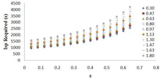
**Figure 8--Isp required as a function of  $\epsilon$  (x-axis) and  $C_{D, \text{geom}}$ . (markers). Isp requirements increase as  $\epsilon$  increases.**
