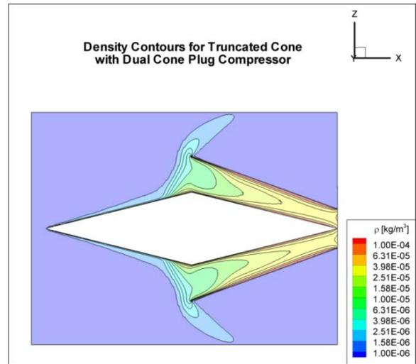
Figure 5--Density contours for truncated cone with compressor.
