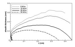
Figure 1: Sheath profile for  $\theta = 60^{\circ}$  magnetic field as a function of normal electric field <sup>2</sup>
