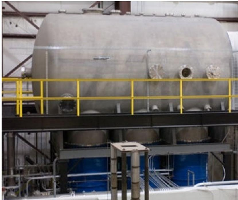
Figure 14. VTF-1 picture showing the blue diffusions pumps below.
