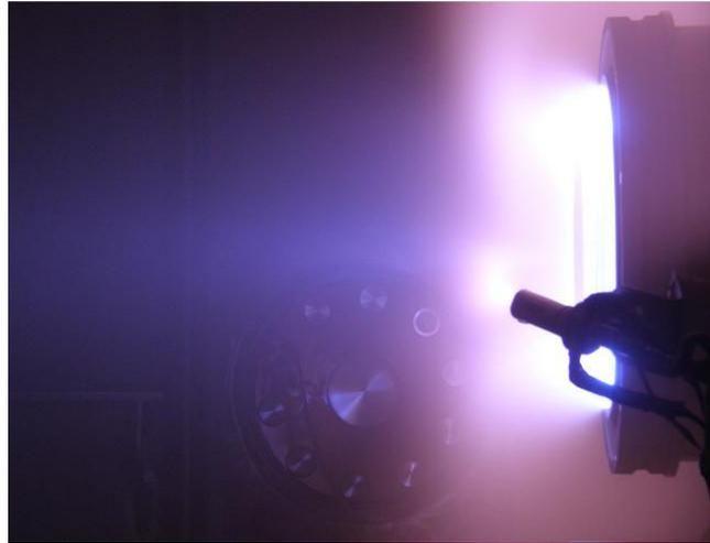
**Figure 43. T-220HT with stainless steel electrodes running on krypton.**
