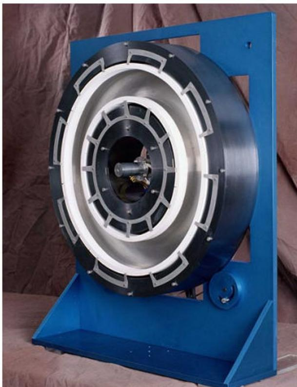
**Figure 6. NASA-457M Hall thruster. The annular anode covers the rear plane and extends along the channel walls. Propellant injection occurs at holes along the inner and outer walls of the annular anode.[30]**
