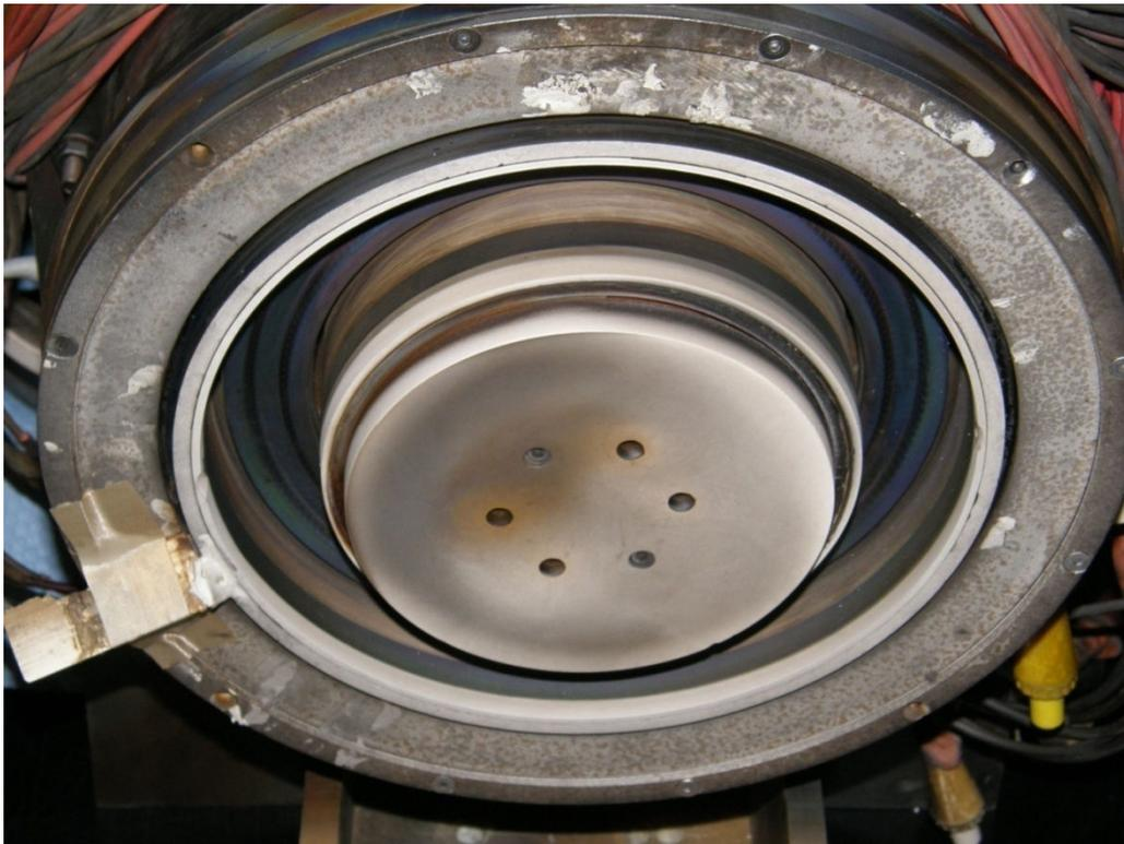
Figure 50. EEHET post test. The white block on the right of the thruster (left side of picture) is a protective cover for the outer electrode wires.
