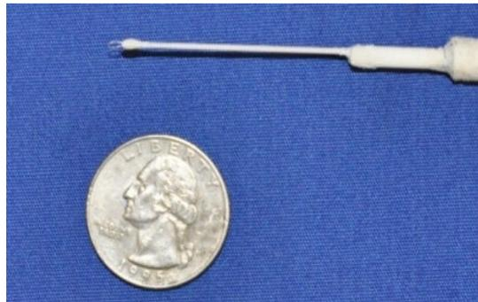
**Figure 33. Miniature emissive probe.**
