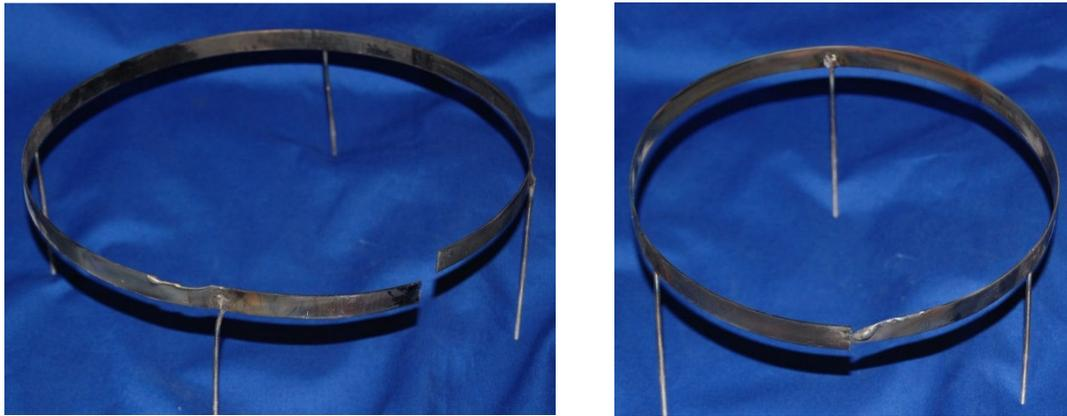
**Figure 36. The stainless steel outer (left), and inner electrodes (right). The electrodes are made from strips of steel and curved to the proper diameter. Steel threaded rods are welded for electrical connections.**
